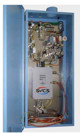
Evaporator system first mixes liquid and carrier gas to easily evaporable aerosol form. Both liquid and carrier gas flows are precisely controlled with mass flow controllers. Aerosol is subsequently evaporated at elevated temperature. Various mixtures can be evaporated, even solids, dissolved in solvents can be vaporized successfully.
