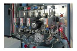
SVCS manufactures individually customized CVD processing system with additional tools to make the R&D system turn-key delivery. The supporting equipment starts from gas cabinets with optional automatic change-over function for uninterrupted gas delivery, followed by gas panels for inert or purging gases.
